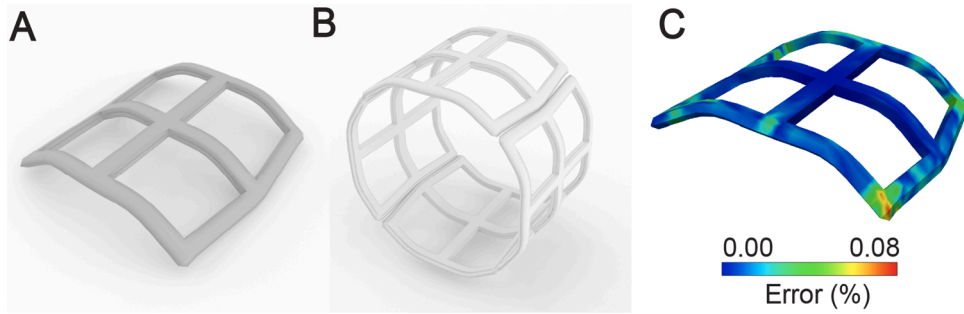
Fig. 9. (A) 2 \times 2 grid in arm band design; (B) arm band; and (C) error distribution of arm band design between prediction and ground truth.
