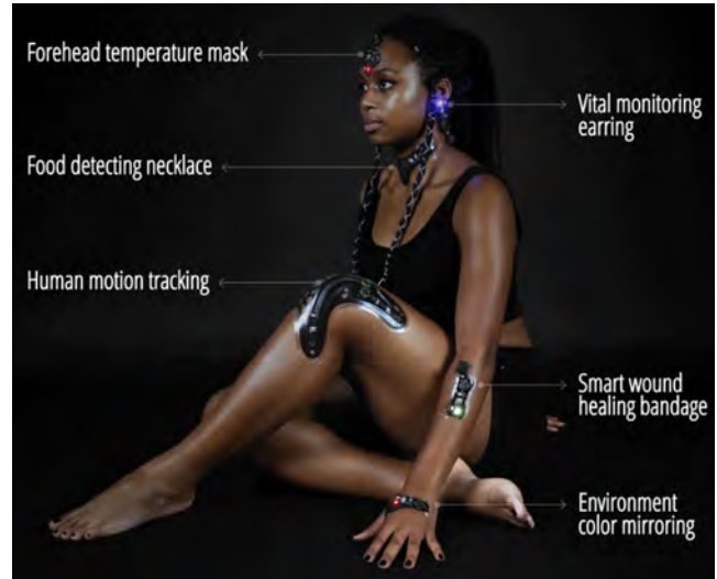
Figure 1: We present ElectroDermis a holistic fabrication approach for fully untethered, stretchable, and on-skin compliant wearable electronics. Here, we show several example applications, including a temperature mask, vital monitoring earrings, context-sensitive necklace, motion tracker, wound monitor, and environment-aware bracelet.
