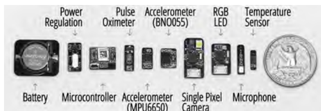
Figure 5. Photograph of the integrated circuit modules, including (left to right) ancillary power management, microcontroller, six digital sensors, and RGB LED.
