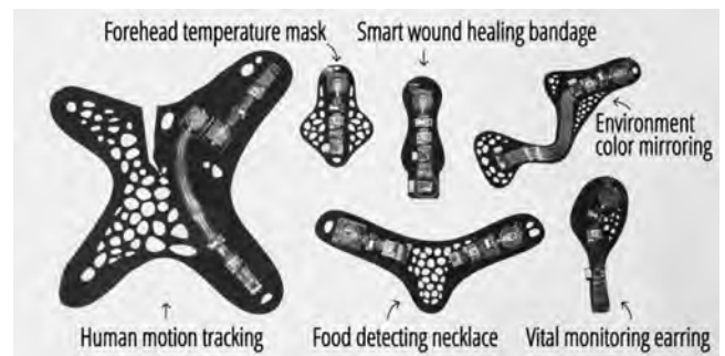
Figure 8: Our ElectroDermis prototypes pre-worn.
