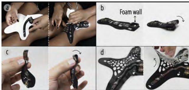
Figure 9: (a) Application of the ElectroDermis. (b) Foam wall used to elevate and prevent the camera from contacting the skin in the smart wound healing bandage. (c) Folding of the vital monitoring earring to allow the pulse oximeter to face the skin. (d) Removal of the skin adhesive for reuse.
