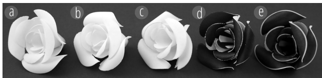
Figure 18. Five roses printed by Thermorph show a good reproducibility. Triggering temperature was 70°C, heating duration was 15 seconds. Mismatch.
