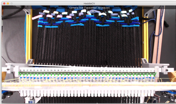
(b) The view from the camera. Green lines show the computer vision's region of interest for each heddle slider.
