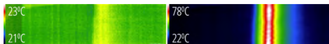
Figure 7: Thermal images of the thick actuator sample before being heated (left) and after it reaches its maximum temperature (right).
