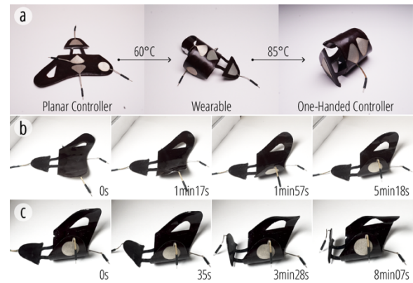
Figure 20: Fabricated shape-changing input device a) in three modes: planar, wearable, and one-handed controller (from left to right). b) The device’s transformation from planar to the wearable controller and c) from the wearable to the one-handed controller.
