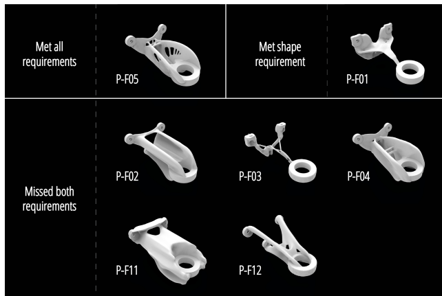
Figure 4: Overview of engine bracket designs created by participants. P-F05 met both the shape and structural requirements. P-F01 only met the shape requirements (the bracket has holes for bolts with sufficient clearance and respects the specified dimensions but is structurally too weak). All other brackets missed both requirements and were either too heavy, weak, larger than the specified dimensions, or had not enough bolt clearance. For simplicity, we only show one design option per participant. Please see the Appendix for all submitted design options.
