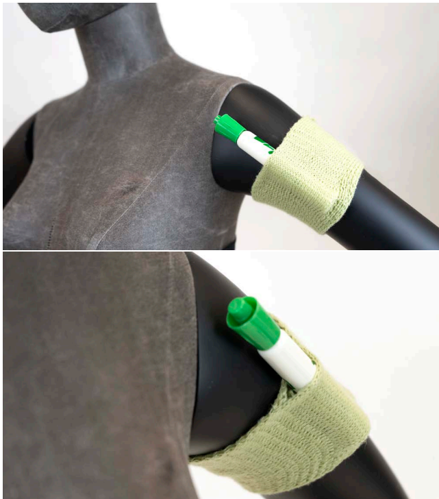
Figure 9: To produce open pockets, the knitter must switch the carriage cam settings every other row, and the rack setting every row. Our system helps the knitter keep track of these.
