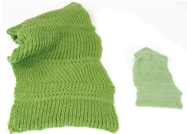
Figure 7: Because we track the machine operations, we can “replay” them on any Knitout-compatible machine. In this case, we have knit a duplicate scarf on a Shima Seiki SWG091N2, which has a much smaller stitch size than our system’s machine.
