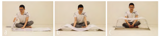
Figure 9. Self-Deforming Furniture: (a) Flexible surface. (b) Self-actuated and deformed. (c) Table becomes stiff by Jamming.
