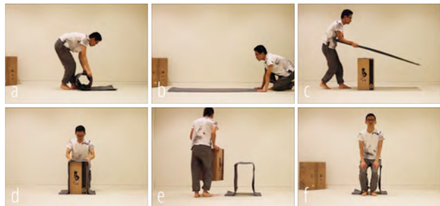
Figure 8. Deformable Furniture: (a) Unwrapping a flexible carpet. (b) Vacuuming the carpet. (c) Carpet becoming stiff. (d) Carpet becoming soft again and conformed to the shape of the box. (e) Carpet turning into a chair. (f) The chair holds weight up to 55kg.
